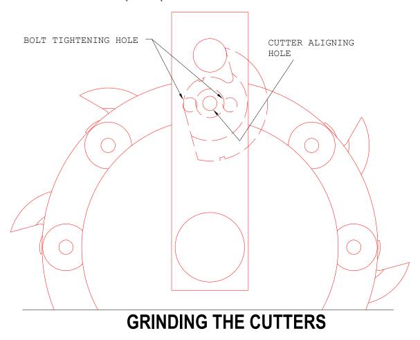
**Grinding the cutters correctly** is a very important factor in obtaining a good fingerjoint. The cutters must always be ground so that the face bevel of the cutter matches the grinding template as shown in the figure below. If the cutters are ground to the incorrect face bevel the joint will not fit correctly. ( See section on TROUBLESHOOTING.)
