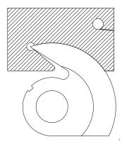
Always check the bevel of the cutters against the **grinding template** as shown above. Cutters ground too blunt (left) or too sharp (right) will produce a weak joint. (See TROUBLESHOOTING section on following page.)
