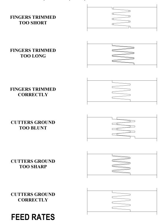
**RPM of the head and FPM** (feet per minute) of the stock both combine to give the measurement known as KMPI (knife marks per inch). Too many KMPI will burn or glaze the wood; leading to premature dulling of the cutters and possibly failure of the glued joint. On the other hand, too few KMPI can lead to too rough a finish or tearout. The knowledgeable operator can fine tune the KMPI to achieve the best quality cut and the longest run times between sharpenings.
