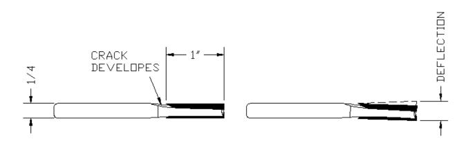
• Low O.D. Clearance/Drag: Deflection of the tool during the cutting process can also lead to severe drag, increased tool pressure, and high cutting temperatures by permitting the O.D. relief portion of the tool to run against the surface just machined, causing overheating and premature cutting edge wear.
